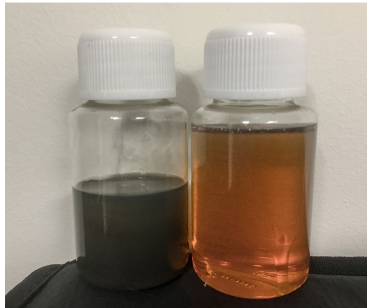
Filtered (right) vs. unfiltered (left) oil.
