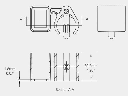
Designed to snap on to a 22.2mm (7/8") diameter handle bar, with a 7.2mm/7.5mm (0.28/0.29") diameter drilled or punched mounting thru hole.
