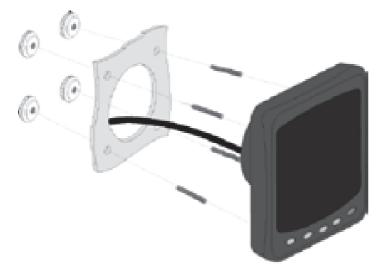
The front mounting kit (M4 studs and thumbnuts) supplied with KAntrak<sup>™</sup>, which allows the display to be mounted onto a panel or vehicle dashboard.
