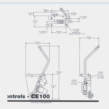
When moving lever from *Disengage* to *Engage* position, the cable travel take up **Mounting 1011001 28** m or 3.60"; the lever travel is 136.7mm or 5.38". Note: If engine is turned off while lever is in *Engage* position, the unit can not
